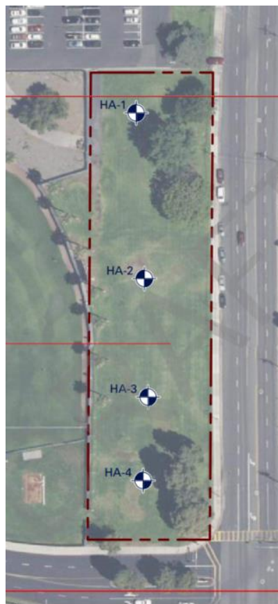
Image 2. Subsurface Hand Auger Locations at Proposed New Parking Lot (Langan 2022, Figure 9).
